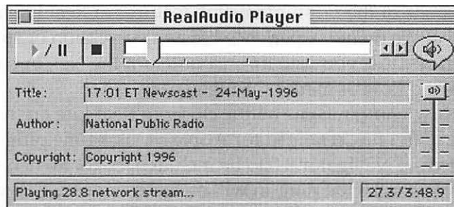
Figure 8-18: The RealAudio Player control panel from which you can start and stop play, adjust volume, and monitor progress of the audio message.
